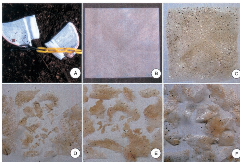
Fig. 3. Composting test of Biomax® films inoculated with isolates.
